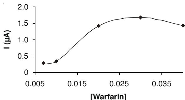
Fig. 8. Effect of concentration of template in the polymerization solution on the peak current of differential pulse voltammograms  $5 \times 10^{-6}$  M warfarin sodium. The other conditions are similar to those illustrated in Fig. 2
