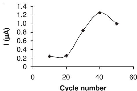
Fig. 5. Influence of the applied number of cyclic scans of polymerization in the reduction signal of entrapped template. All conditions are similar to those illustrated in Fig. 2.
