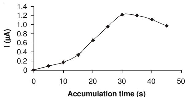
Fig. 6. Influence of the accumulation time period on the peak current of differential pulse voltammograms for  $5 \times 10^{-6}$  M warfarin sodium. The other conditions are similar to those illustrated in Fig. 2
