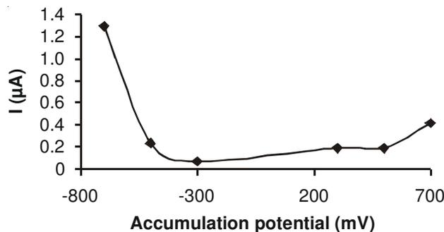
Fig. 7. Effect of accumulation potential on the peak current of differential pulse voltammograms for  $5 \times 10^{-6}$  M warfarin sodium. The other conditions are similar to those illustrated in Fig. 2
