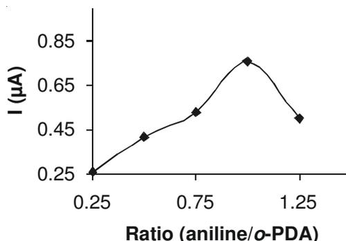
Fig. 3. Reduction signal of the entrapped template in MIP electrode after being synthesized with different *o*-PDA: aniline ratios. The other conditions are similar to those illustrated in Fig. 2
