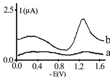
Fig. 2. Differential pulse voltammograms corresponding to the reduction signal of the entrapped template measured by (a) a MIP electrode after extracting the template (b) a MIP electrode after accumulation of  $5 \times 10^{-6}$  M warfarin sodium in a Britton-Robinson buffer (pH = 2.0) for 60 s at -700 mV accumulation potential. Measurements made in a Britton-Robinson 0.04 M buffer solution of pH 2.0 at a scan rate of 100 mV/s. Pulse amplitude = 50 mV, pulse width = 40 ms
