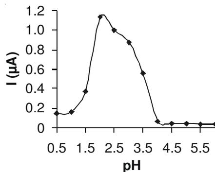
Fig. 4. Effect of pH of measurement solution on the peak current of differential pulse voltammograms for  $5 \times 10^{-6}$  M warfarin sodium. The other conditions are similar to those illustrated in Fig. 2
