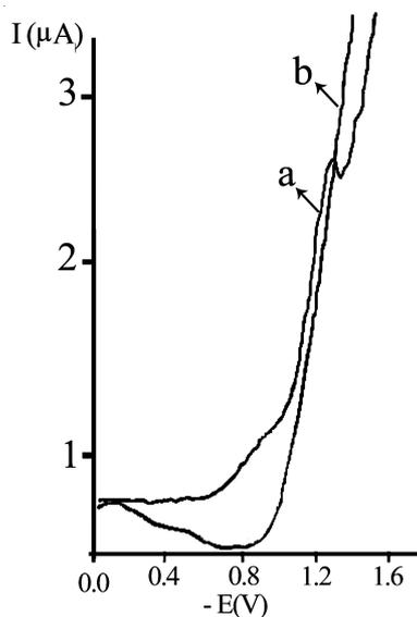
Fig. 1. Differential pulse voltammograms for  $5 \times 10^{-6}$  M warfarin sodium in a B-R buffer (pH = 5.0) with pre-concentration time of 30 s in -0.7 V pre-concentration potential at scan rate of 100 mV/s; at (a) HMDE and (b) Bi-film electrode. Pulse amplitude = 50 mV, pulse width = 40 ms
