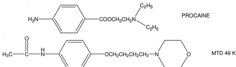
Fig. 2. Chemical structures of procaine and MTD 46 K
