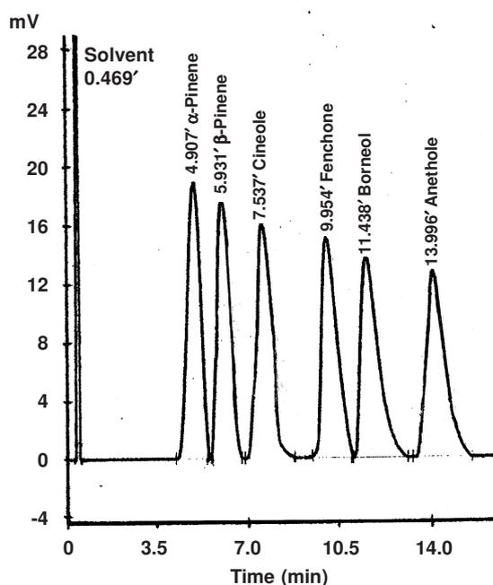
Fig. 4. Chromatogram for some essential oils (column 2 m  $\times$  2 mm packed with modified chromosorb G, programmed temperature 35-125 °C with increasing rate 6 °C/min, flow rate of N<sub>2</sub> 40 mL/min, the injection volume 0.2  $\mu$ L and injected port temperature 175 °C)
