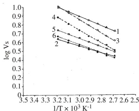
Fig. 2. Variation of  $\log V_s = f(1/T)$  on (2 m × 2 mm) packed columns using free chromosorb G (1,3,5) and grafted chromosorb G (2,4,6): 1,2-*n*-pentan, 3,4-benzene, 5,6-dichloromethane
