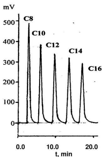
Fig. 5. Chromatogram of standard mixture of fatty acids (C8, C10, C12, C14 and C16) as methyl esters (GLC-30) (column 2 m × 2 mm packed with modified chromosorb G, programmed temperature 90-235 °C with increasing rate 6 °C/min, flow rate of N<sub>2</sub> 40 mL/min, the injection volume 0.2 μL and injected port temperature 250 °C)
