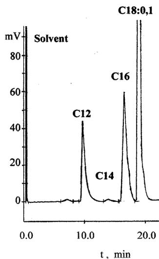
Fig. 7. Chromatogram of extracted laurel oil from fruit of cultivated *laurius nobilis* (column 2 m  $\times$  2 mm packed with modified chromosorb G, programmed temperature 90-235  $^{\circ}$ C with increasing rate 6  $^{\circ}$ C/min, flow rate of  $N_2$  40 mL/min, the injection volume 0.2  $\mu$ L and injected port temperature 250  $^{\circ}$ C)
