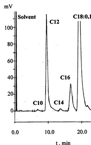
Fig. 6. Chromatogram of laurel oil extracted from wild fruit of *Laurus nobilis* (column 2 m × 2 mm packed with modified chromosorb G, programmed temperature 90-235 °C with increasing rate 6 °C/min, flow rate of N<sub>2</sub> 40 mL/min, the injection volume 0.2 μL and injected port temperature 250 °C)
