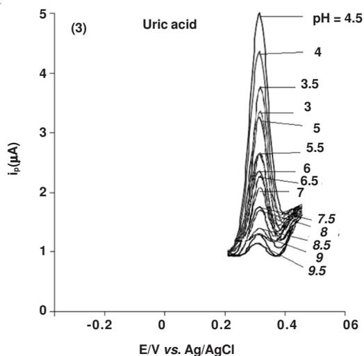
Fig. 5 Variation of peak current value of differential pulse voltammetry in different pH for oxidation of 3 mM ascorbic acid (AA), 100  $\mu M$  dopamine (DA) and 200  $\mu M$  uric acid (UA). Scan rate is 50 mV/s in room temperature
