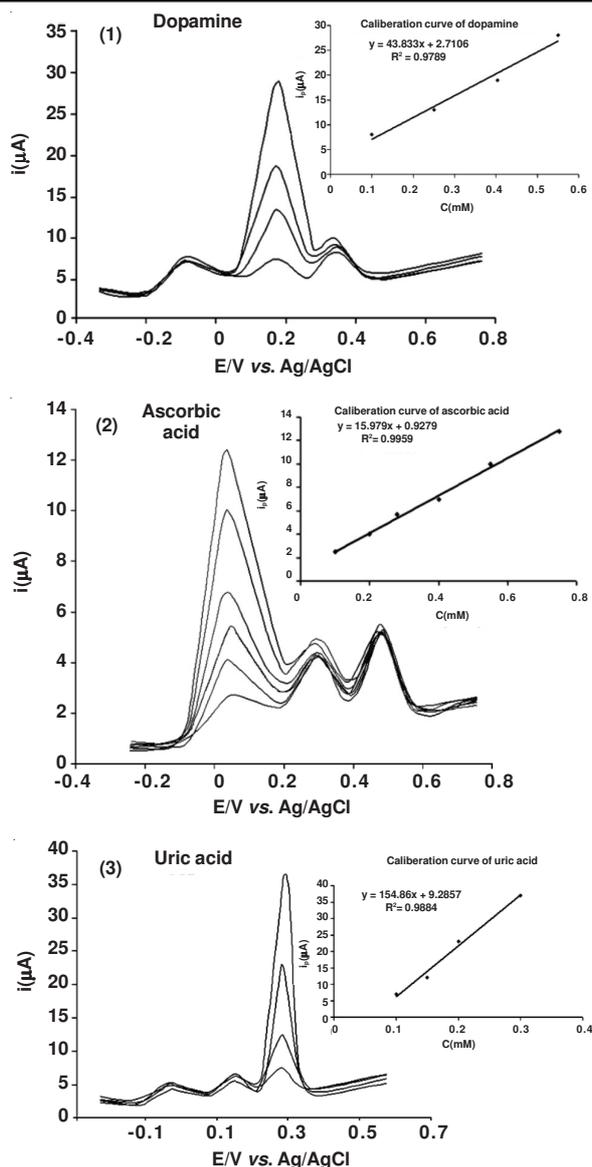
Fig. 8. Differential pulse voltammetry (DPV) of dopamine (DA), ascorbic acid (AA) and uric acid (UA) in different concentration on glassy carbon electrode (GCE) and ionic liquid glassy carbon electrode in phosphate buffer in room temperature and 2 mm electrode diameter. Other species in each measuring is 0.1 mM
