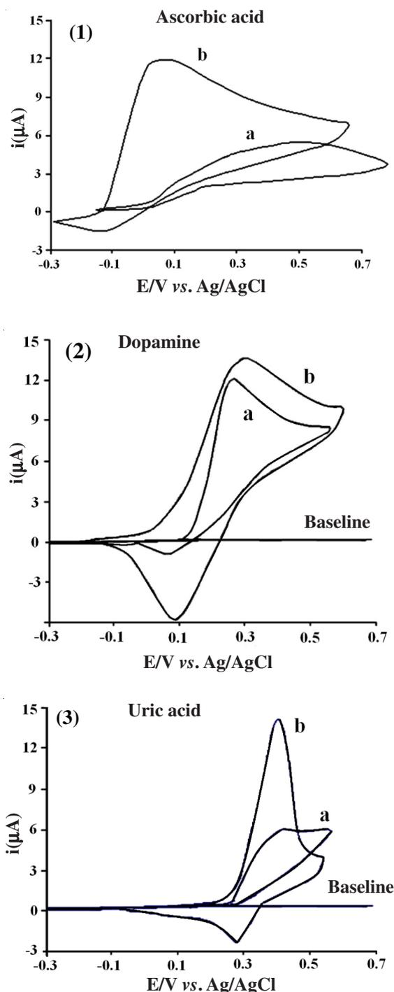
Fig. 3. Cyclic voltammograms of 4 mM of dopamine (DA), ascorbic acid (AA) and uric acid (UA) on (a) glassy carbon electrode (GCE) and (b) Ionic liquid glassy carbon electrode (ILGCE). Scan rate is 50 mV/s and pH of phosphate buffer is 7
