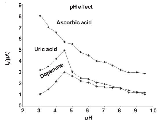
Fig. 6 Investigation of variation of peak current value with pH for oxidation of 3 mM ascorbic acid (AA), 100  $\mu M$  dopamine (DA) and 200  $\mu M$  uric acid (UA). Scan rate is 50 mV/s in room temperature
