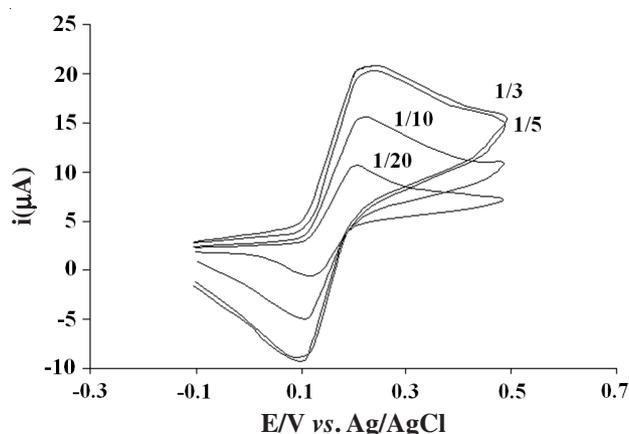
Fig. 1. Cyclic voltammogram of 2  $\mu$ M of dopamine (DA) on modified glassy carbon electrode (GCE) in different w/w ratio of [omim]PF<sub>6</sub> in acetonitrile. Scan rate is 50 mV/s and glassy carbon electrode diameter is 2 mm
