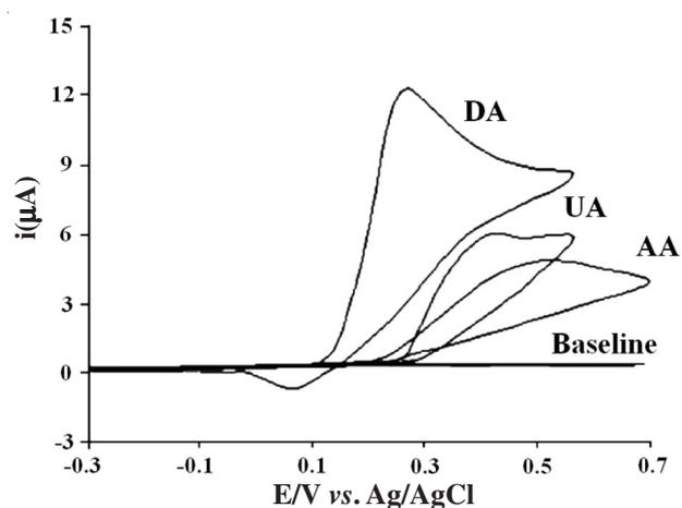
Fig. 2. Cyclic voltammograms of 4 mM of dopamine (DA), ascorbic acid (AA) and uric acid (UA) on glassy carbon electrode (GCE). All the peaks were overlaid. Scan rate is 50 mV/s and pH phosphate buffer is 7
