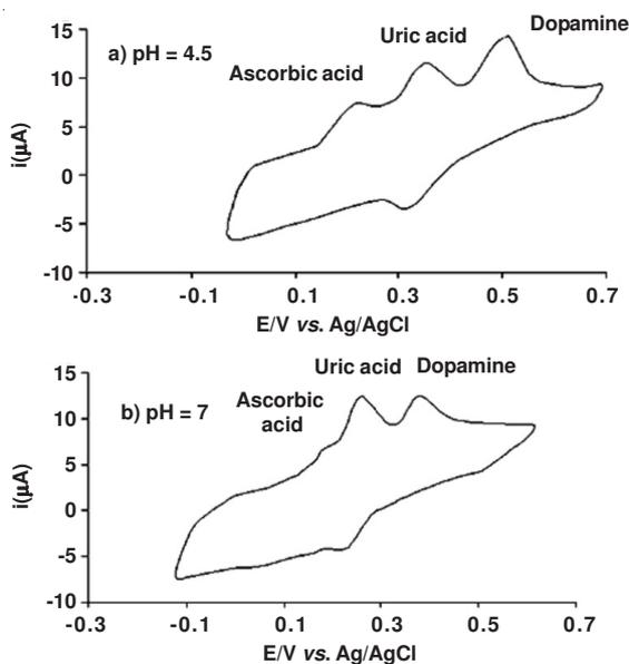
Fig. 7 Cyclic voltammogram of mixture of dopamine (DA), uric acid (UA) and ascorbic acid (AA) in 2 mM concentration and 10 mM phosphate buffer in pH 4.5 and 7. Scan rate is 50 mV/s and temperature is 18  $^{\circ}C$
