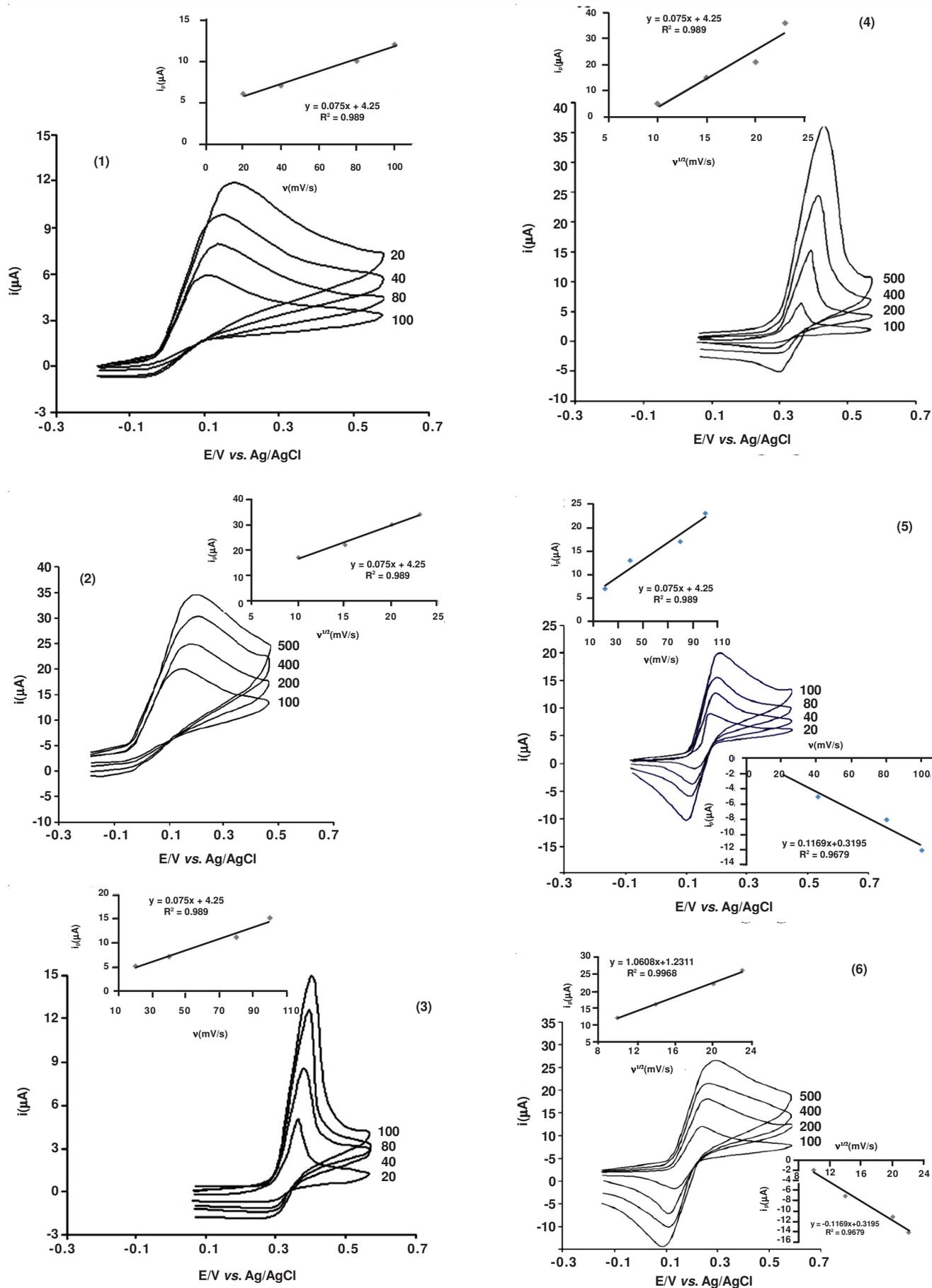
Fig. 4. Scan rate effect and its calibration curve for ascorbic acid, uric acid and dopamine in 2 mM concentration in two ranges 20-100 and 100-500 is shown. Buffer is phosphate with pH = 4.5
