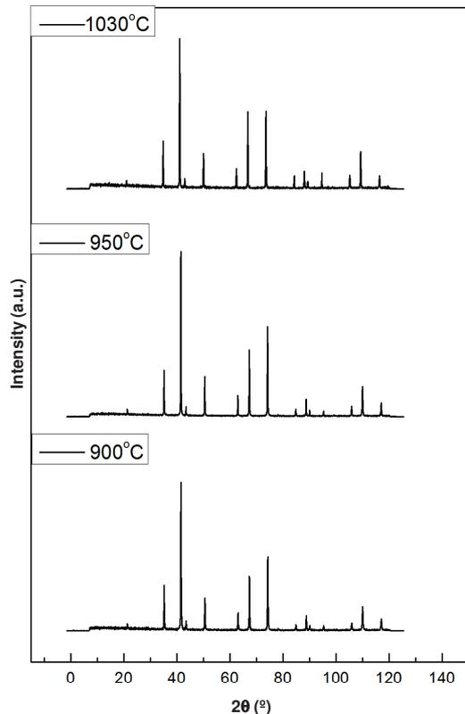
Fig. 1. XRD patterns of the sintered samples
