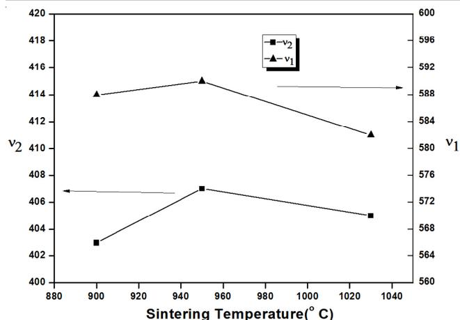
Fig. 2. Variation of  $v_1$ ,  $v_2$  with sintering temperature
