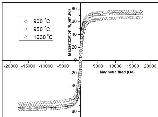
Fig. 3. Room temperature hysteresis loops for sintered samples
