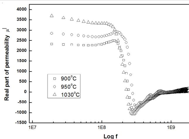
Fig. 4. Real part of permeability with frequency for sintered samples
