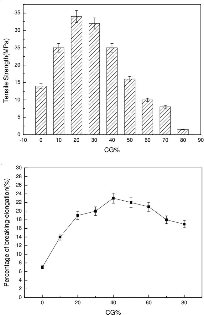
Fig. 4. Dependence of tensile strength and the elongation at break on the content of *Grifola frondosa* for the blend films
