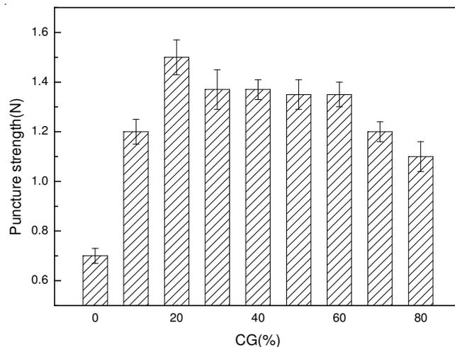
Fig. 5. Dependence of puncture strength on the content of *Grifola frondosa* for the blend films
