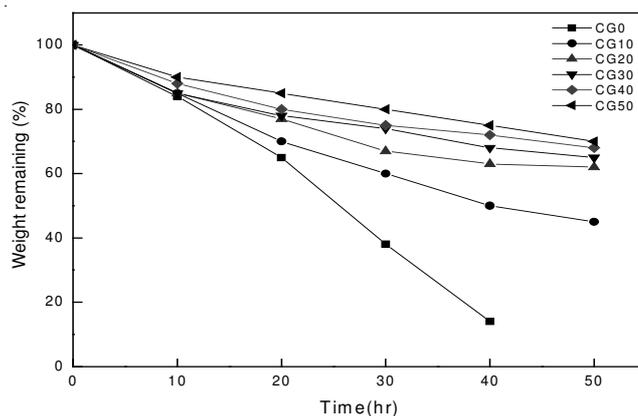
Fig. 7. *In vitro* degradation of chitosan and blend films in 4 mg mL<sup>-1</sup> lysozyme solution of pH 7.4 at 37 °C
