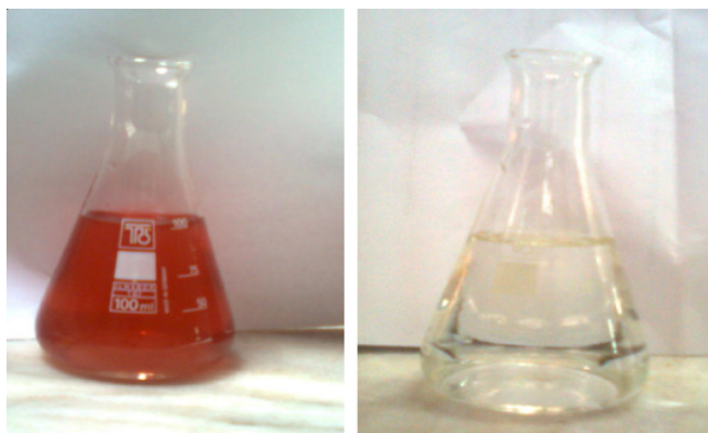
Fig.1. Solutions of silver nitrate (0.001 M) before (right) and after (left) exposure to the culture filtrate of E. coli
