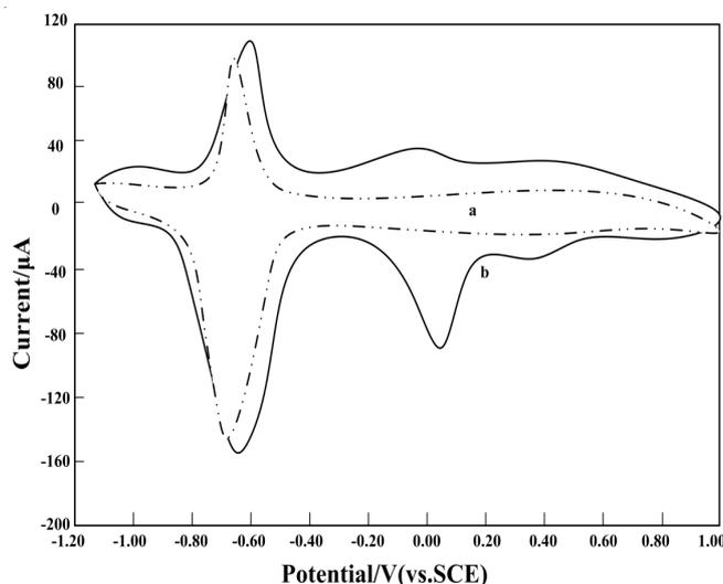
Fig. 2. Cyclic voltammograms of 0.01 M acetate buffer (pH 6.0) containing (a) 0.8  $\mu M$  In(III) and 0.6  $\mu M$  Al(III); (b) (a) + 40  $\mu M$  eriochrome blue black R, with scan rate of 100 mV s<sup>-1</sup>
