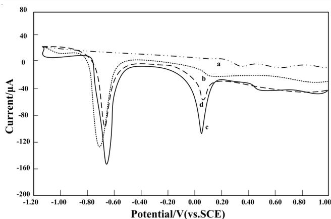
Fig. 3. Adsorptive stripping voltammograms of: (a) 40  $\mu\text{M}$  of eriochrome blue black R solution at pH 6.0 after 30 s accumulation time at -1.0 V; (b) 0.8  $\mu\text{M}$  In(III) and 0.6  $\mu\text{M}$  Al(III) under similar experimental conditions as (a); (c) (a) + (b) under similar experimental conditions as (a); and (d) solution (c) without accumulation time, with scan rate of 100  $\text{mV s}^{-1}$
