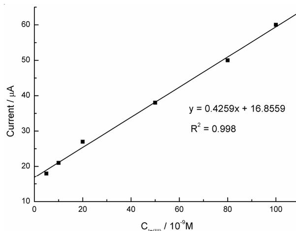
Fig. 8. Calibration plot of In(III) in the presence of 0.1  $\mu\text{M}$  aluminum ion at optimum conditions (pH = 6.0, EBBR = 40  $\mu\text{M}$ , accumulation potential = -1.0 V, accumulation time = 30 s and scan rate = 100  $\text{mV s}^{-1}$ )
