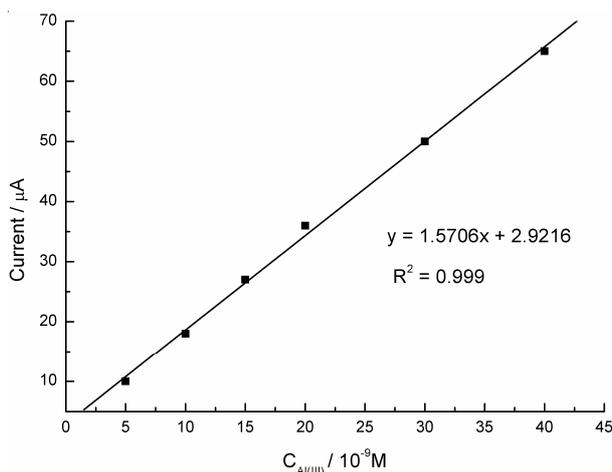
Fig. 9. Calibration plot of Al(III) in the presence of 0.1  $\mu\text{M}$  indium ion at optimum conditions (pH = 6.0, EBBR = 40  $\mu\text{M}$ , accumulation potential = -1.0 V, accumulation time = 30 s and scan rate = 100  $\text{mV s}^{-1}$ )
