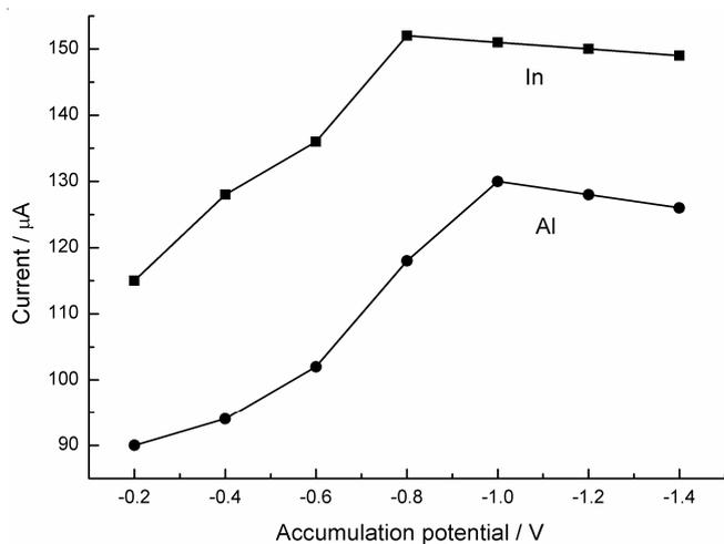
Fig. 6. Effect of accumulation potential on the stripping peak currents of 0.8  $\mu\text{M}$  In(III) and Al(III) in the presence of 40  $\mu\text{M}$  EBBR. Other conditions as in Fig. 5
