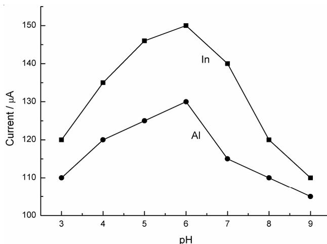
Fig. 4. Effect of pH on the stripping peak currents of 0.8  $\mu\text{M}$  In(III) and Al(III) in the presence of 40  $\mu\text{M}$  EBBR and after 30 s accumulation time at -1.0 V
