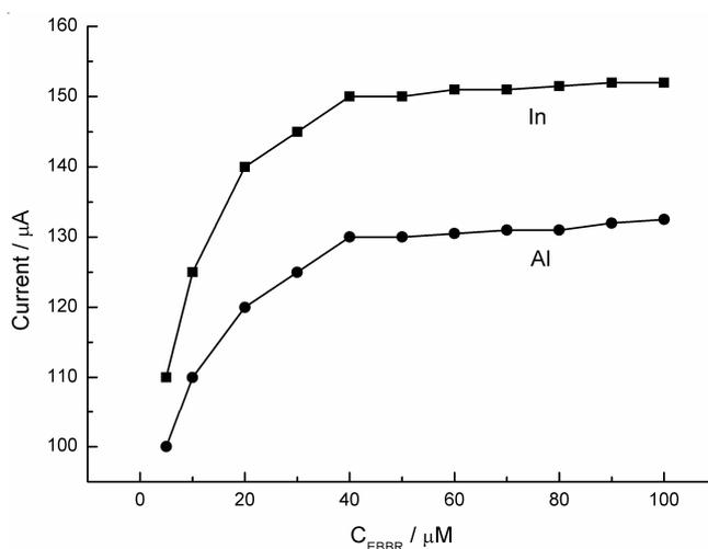
Fig. 5. Effect of EBBR concentration on the stripping peak currents of 0.8  $\mu\text{M}$  In(III) and Al(III) at pH 6.0. Other conditions as in Fig. 4
