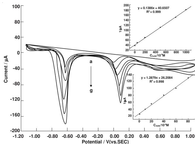
Fig. 10. Adsorptive stripping voltammograms of different concentrations of In(III) and Al(III): (a) 0, 0 µM, (b) 0.005, 0.010 µM, (c) 0.050, 0.100 µM, (d) 0.200, 0.200 µM, (e) 0.500, 0.400 µM, (f) 0.800, 0.600 µM and (g) 1.000, 0.800 µM, respectively, at optimal conditions (pH = 6.0, EBBR = 40 µM, accumulation potential = -1.0 V, accumulation time = 30 s and scan rate = 100 mV s<sup>-1</sup>)
