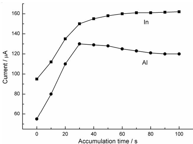
Fig. 7. Effect of accumulation time on the stripping peak currents of 0.8  $\mu\text{M}$  In(III) and Al(III) at -1.0 V. Other conditions as in Fig. 6
