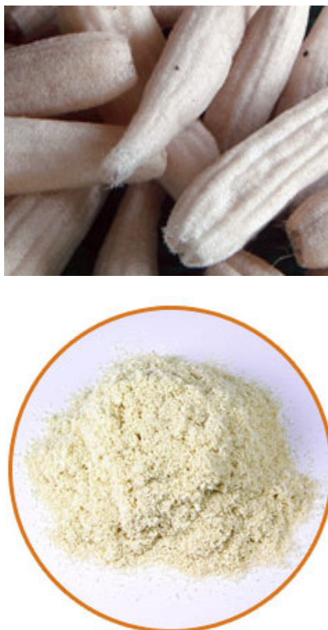
Fig 1. (a) Luffa fruits fibers (b) grounded fibers (pulp) distinctive with its whitish colour
