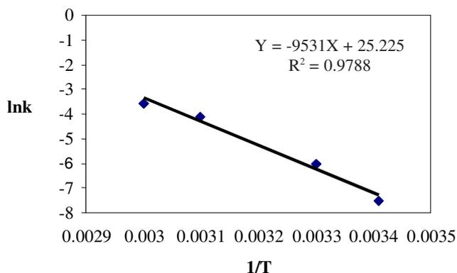
Fig. 8. Plot of Arrhenius for the adsorption of reactive dye methyl orange onto biosorbent (tail of black cherry)
