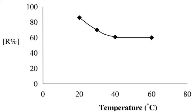
Fig. 5. Effect of temperature on the removal of methyl orange onto biosorbent tail of black cherry. Conditions: initial concentration 150 mg/L; adsorbent 0.1g; temperatures (20, 30, 40, 60 °C)
