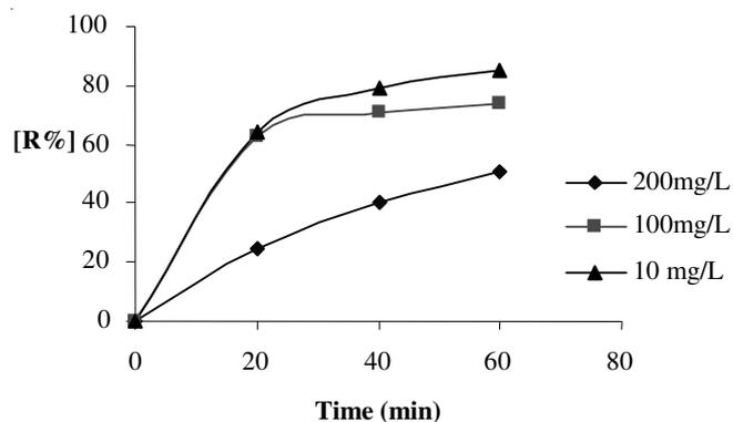
Fig. 2. Effect of contact time on the removal of reactive dye at different initial concentrations onto tail of black cherry. Conditions: adsorbent 0.1g; contact time 1 h
