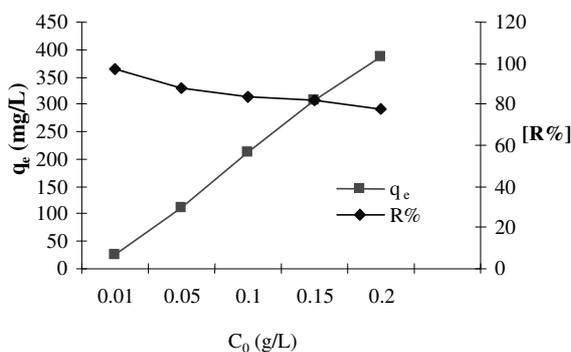
Fig. 1. Effect of initial concentrations on the removal of reactive dye methyl orange onto activated carbon (tail of black cherry)
