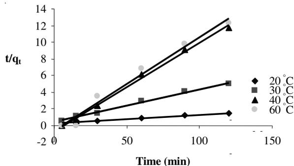
Fig. 7. Plot of pseudo second-order models to reactive dye methyl orange sorption onto tail of black cherry in an initial concentration 50mg/L; adsorbent 0.1g; contact time 2 h
