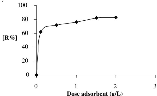
Fig. 3. Effect of biosorbent dose tail of black cherry on the removal of reactive dye methyl orange. Conditions: initial concentration 50 mg/L; temperature 25 °C; contact time 1 h.
