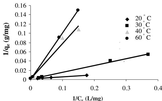
Fig. 6. Plot of Langmuir for the adsorption of the reactive dye methyl orange onto activated carbon tail of black cherry at different temperatures.
