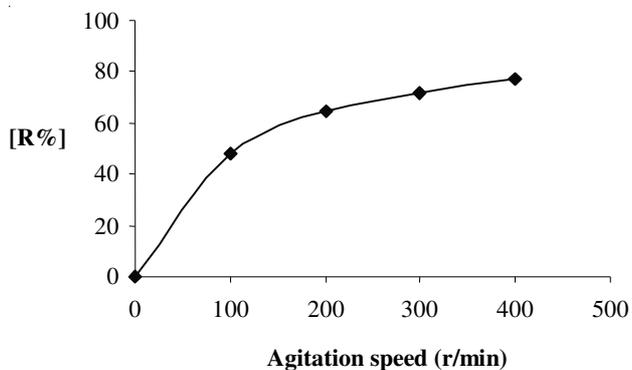
Fig. 4. Effect of agitation speed on the adsorption reactive dye methyl orange onto tail of black cherry. Conditions: initial concentration 50 mg/L; adsorbent 0.1 g; contact time 3 h
