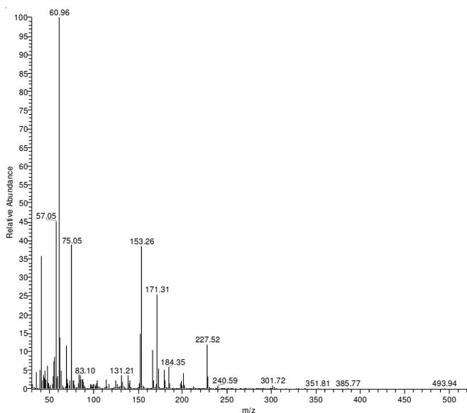
Fig. 2. Mass spectrum of <sup>15</sup>N-methionine trifluoroacetyl butyl ester, M = 228
