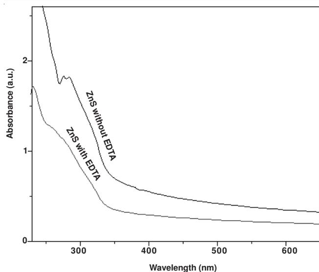
Fig. 3. Absorption spectrum of Mn<sup>2+</sup> doped ZnS nanoparticles
