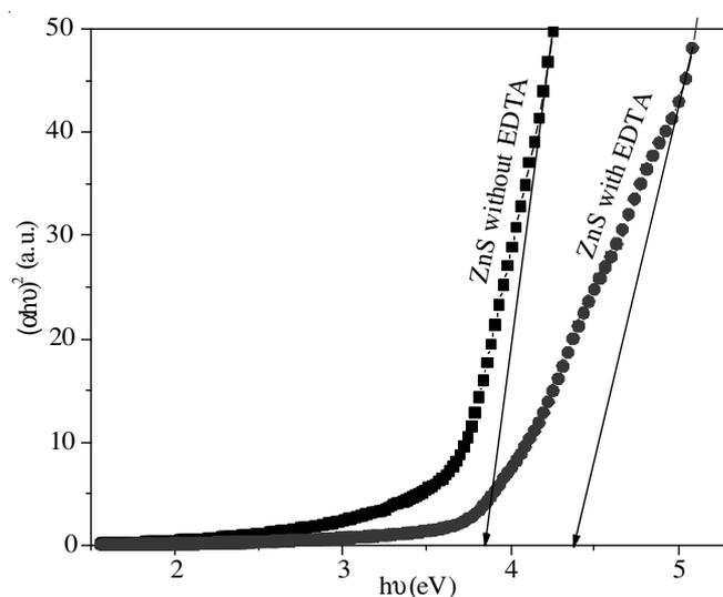
Fig. 4. Calculation of the band gap energy from the UV-VIS absorption spectra
