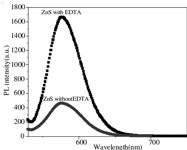
Fig. 5. Show the PL emission from the ZnS:Mn nanoparticle
