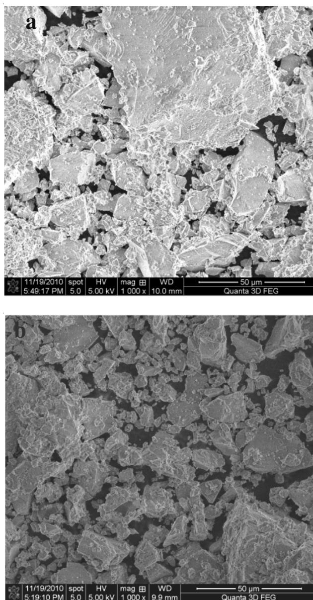
Fig. 2. FESEM image of (a) ZnS:Mn without EDTA (b) ZnS:Mn with EDTA
