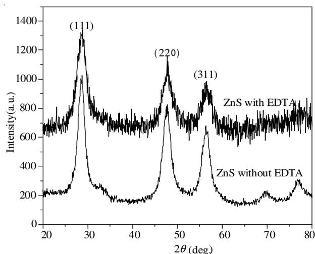
Fig. 1. XRD pattern of ZnS:Mn nanoparticle
