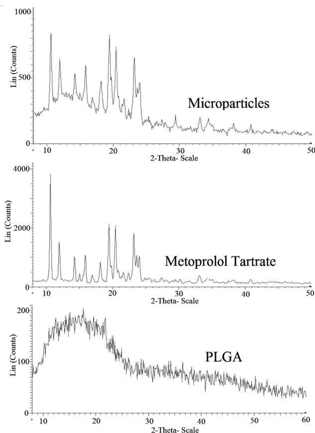
Fig. 4. XRD profiles of PLGA, MT and MT-loaded PLGA microparticles
