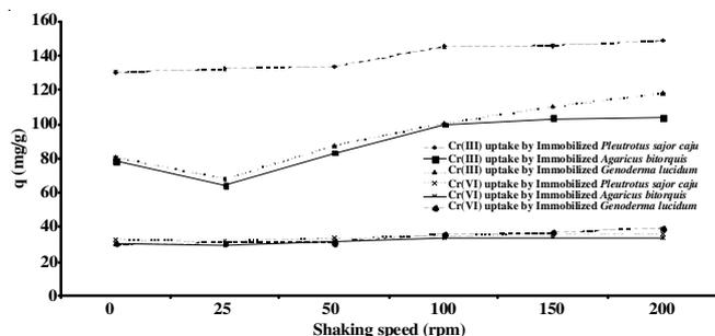
Fig. 7. Effect of shaking speed on Cr(III) and Cr(VI) uptake by immobilized white rot fungi
