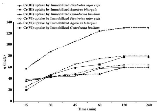
Fig. 5a. Effect of time on Cr(III) and Cr(VI) uptake by immobilized white rot fungi at 30 °C
