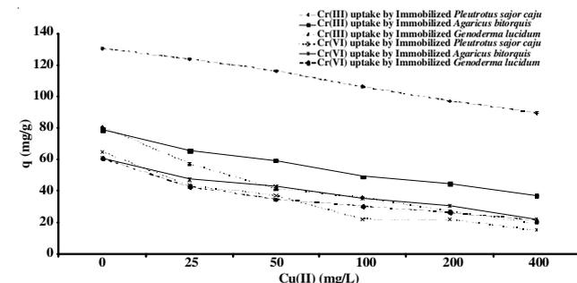
Fig. 8d. Effect of Cu(II) concentration in solution on Cr(III) and Cr(VI) uptake by immobilized white rot fungi
