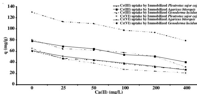
Fig. 8b. Effect of Ca(II) concentration in solution on Cr(III) and Cr(VI) uptake by immobilized white rot fungi
