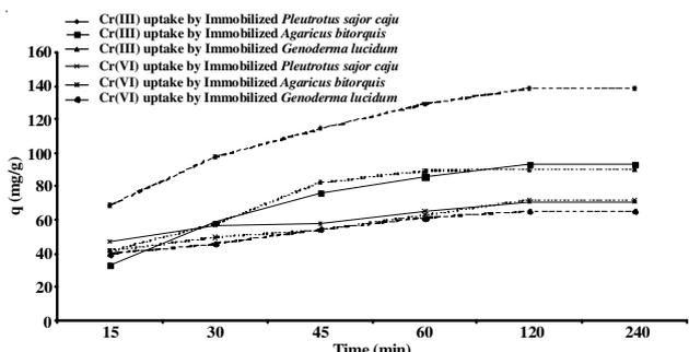
Fig. 5c. Effect of time on Cr(III) and Cr(VI) uptake by immobilized white rot fungi at 50 °C
