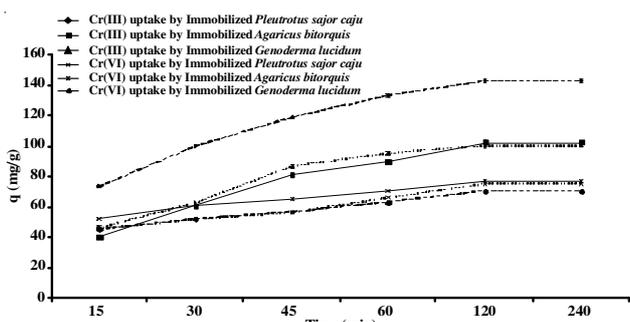
Fig. 5d. Effect of time on Cr(III) and Cr(VI) uptake by immobilized white rot fungi at 55 °C
