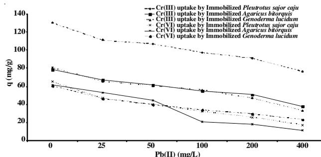
Fig. 8e. Effect of Pb(II) concentration in solution on Cr(III) and Cr(VI) uptake by immobilized white rot fungi
