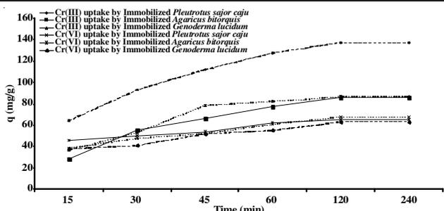
Fig. 5b. Effect of time on Cr(III) and Cr(VI) uptake by immobilized white rot fungi at 40 °C
