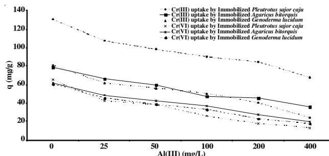
Fig. 8c. Effect of Al(III) concentration in solution on Cr(III) and Cr(VI) uptake by immobilized white rot fungi
