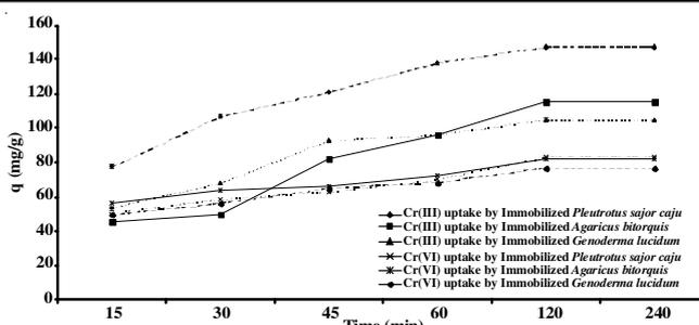
Fig. 5e. Effect of time on Cr(III) and Cr(VI) uptake by immobilized white rot fungi at 60 °C
