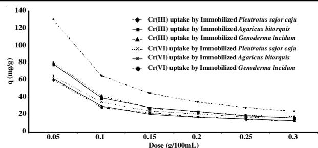
Fig. 3. Effect of biosorbents concentration on Cr(III) and Cr(VI) uptake by immobilized white rot fungi
