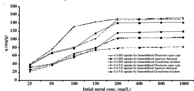
Fig. 4. Effect of initial metal concentration on Cr(III) and Cr(VI) uptake by immobilized white rot fungi
