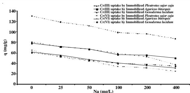
Fig. 8a. Effect of Na concentration in solution on Cr(III) and Cr(VI) uptake by immobilized white rot fungi
