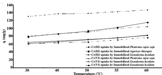
Fig. 6. Effect of temperature on Cr(III) and Cr(VI) uptake by immobilized white rot fungi
