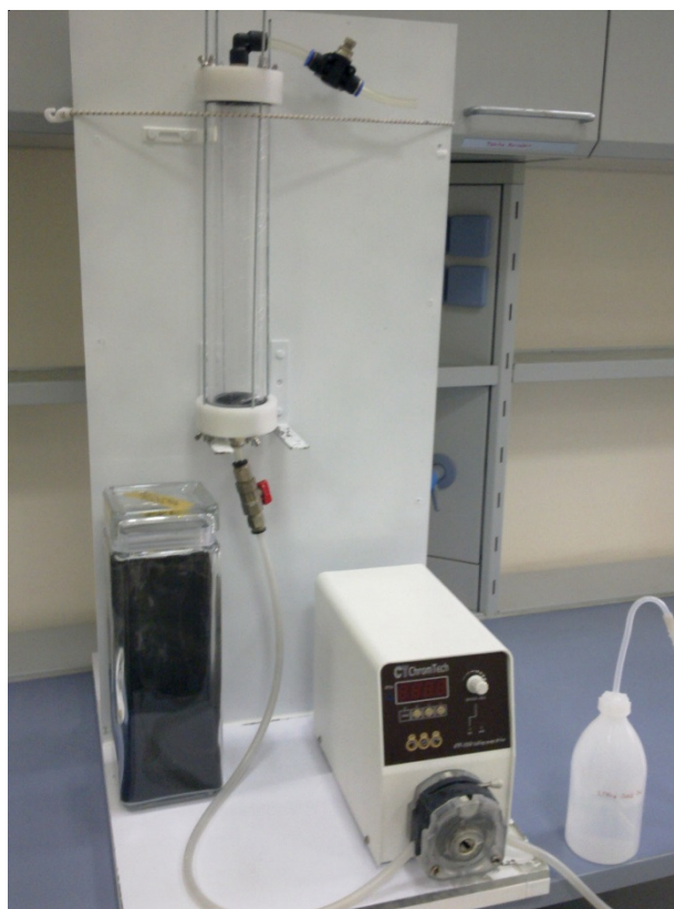
Fig. 1. Experiment device prepared in the laboratory according to ASTM D 4874-95
