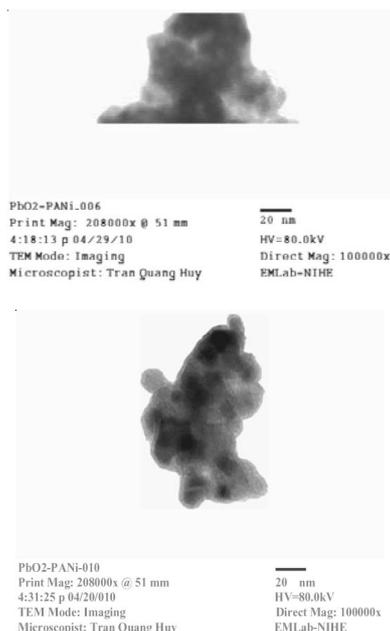
Fig. 5. TEM images of PbO<sub>2</sub>-PANi composites prepared by cyclic voltammetric method with 300 cycles at scan rate of 100 mV/s from acid medium
