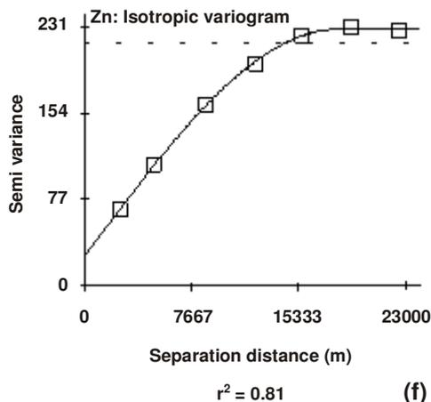
Fig. 3. Experimental semi-variograms for each heavy metals: (a) Cd; (b) Co; (c) Cu; (d) Ni; (e) Pb and (f) Zn
