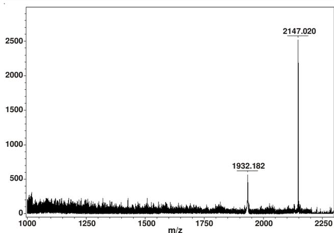
Fig. 5. MALDI mass spectrum of the sulfonated byproduct
