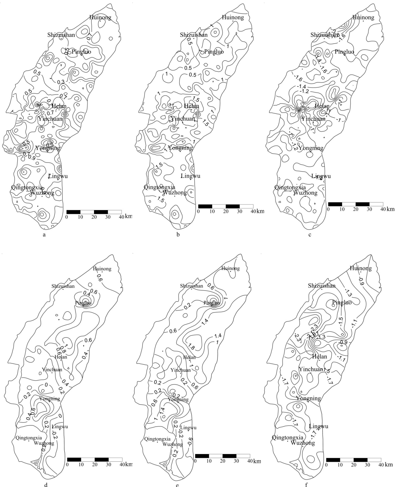
Fig. 13. Contours maps of SI. (a) SI of calcite in phreatic water, (b) SI of dolomite in phreatic water, (c) SI of gypsum in phreatic water, (d) SI of calcite in confined water, (e) SI of dolomite in confined water, (f) SI of gypsum in confined water
