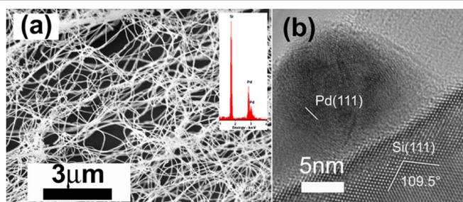
Fig. 2. (a) SEM image of SiNWs and EDX spectrum (inset) of SiNWs supported Pd catalyst; (b) HRTEM image of a single SiNW supported Pd nanostructure
