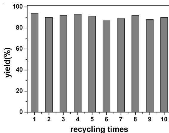
Fig. 3. Recycling of SiNWs supported Pd catalysts for the Heck reaction of iodobenzene with methyl acrylate
