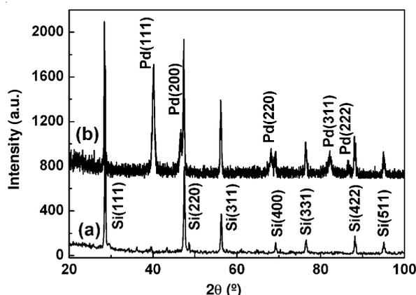
Fig. 1. XRD patterns of (a) SiNWs and (b) SiNWs supported palladium nanostructure.
