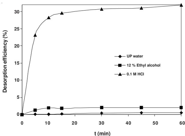
Fig. 9. Methylene blue recovery by different desorbents
