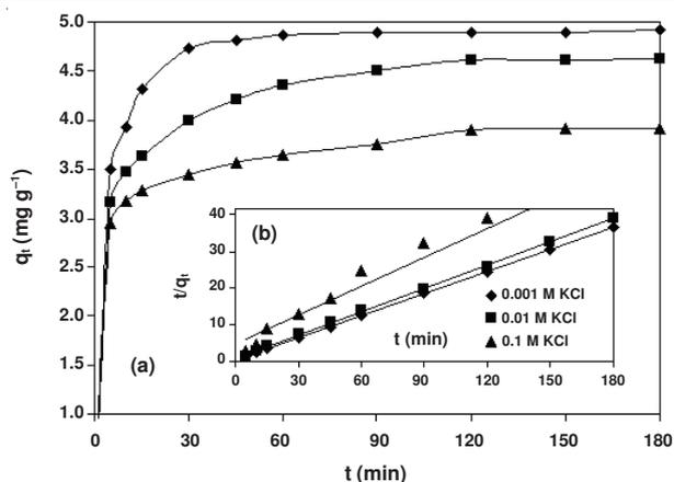
Fig. 8. Effect of ionic strength (a) and pseudo-second-order plots methylene blue onto base activated prina (b) (solid/liquid: 10 g L<sup>-1</sup>, 298 K, natural pH, C<sub>0</sub>: 50 mg L<sup>-1</sup> and stirring speed: 400 rpm)
