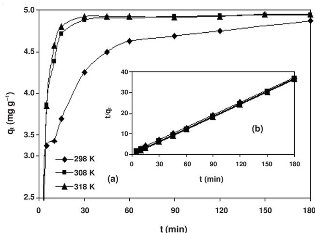
Fig. 7. Effect of temperature (a) and pseudo-second-order plots methylene blue onto base activated prina (b) (solid/liquid: 10 g L<sup>-1</sup>, natural pH, C<sub>0</sub>: 50 mg L<sup>-1</sup>, ionic strength: 0.0 g L<sup>-1</sup> and stirring speed: 400 rpm)
