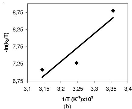
Fig. 10. (a) Arrhenius plot for the adsorption and (b) plot of  $\ln(k_2/T)$  versus  $1/T$  for adsorption of dye on base activated prina
