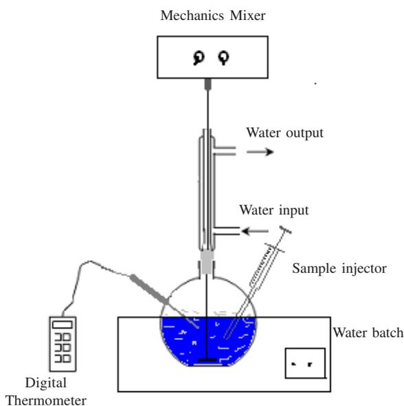
Fig. 2. Reactor of batch process
