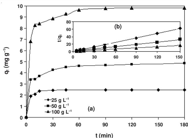
Fig. 5. Effect of initial concentration (a) and pseudo-second-order plots methylene blue onto base activated prina (b) (solid/liquid: 10 g L<sup>-1</sup>, 298 K, natural pH, ionic strength: 0.0 g L<sup>-1</sup> and stirring speed: 400 rpm)
