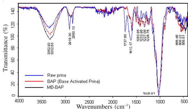
Fig. 3. FTIR spectra belong to raw prina, base activated prina and a methylene blue-base activated prina
