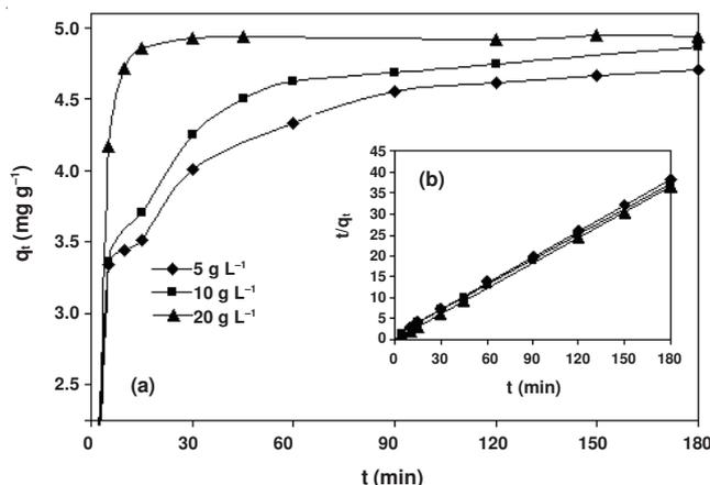
Fig. 4. Effect of adsorbents dosage (a) and pseudo-second-order plots methylene blue onto base activated prina (b) (298 K; natural pH,  $C_0$ :  $50 \text{ mg L}^{-1}$ , ionic strength:  $0.0 \text{ g L}^{-1}$  and stirring speed:  $400 \text{ rpm}$ )
