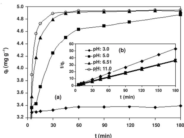
Fig. 6. Effect of pH (a) and pseudo-second-order plots methylene blue onto base activated prina (b) (solid/liquid: 10 g L<sup>-1</sup>, 298 K, C<sub>0</sub>: 50 mg L<sup>-1</sup>, ionic strength: 0.0 g L<sup>-1</sup> and stirring speed: 400 rpm)
