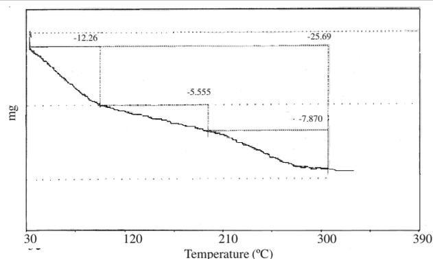
Fig. 2. Thermogravimetric analysis of iron of histidine complex
