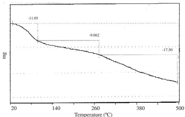
Fig. 4. Thermogravimetric analysis of chromium complex of histidine
