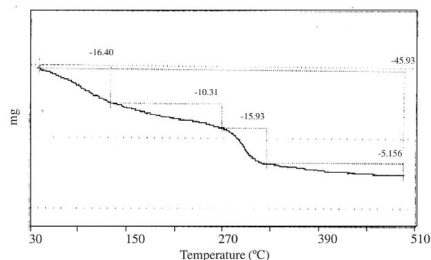
Fig. 3. Thermogravimetric analysis nickel complex of histidine
