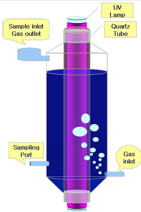
Fig. 1. Photodecomposition test reactor
