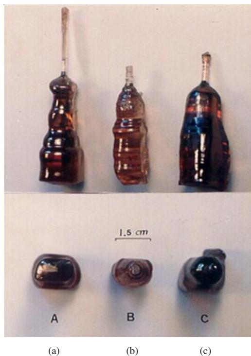
Fig. 5. The grown single crystals of  $ZnWO_4$  in (a) [100], (b) [010] and (c) [001], which corresponds to Table-4 (A), (B) and (C) with the growth direction, rotation speed and diameter
