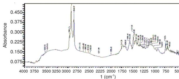
Fig. 8. FTIR spectrum of stearoyl chitosan
