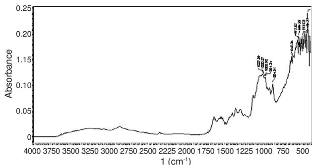
Fig. 2. FTIR spectrum of chitosan
