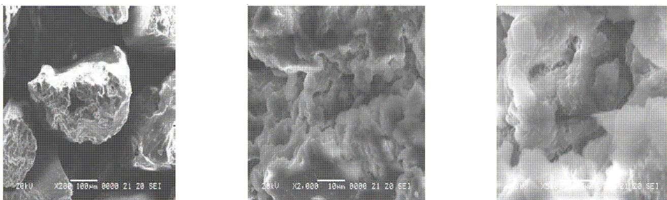
Fig. 18. Scanning electron microscope photograph of decanoyl chitosan
