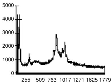
Fig. 15. X-Ray spectrum of stearoyl chitosan
