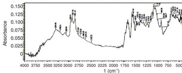
Fig. 4. FTIR spectrum of decanoyl chitosan
