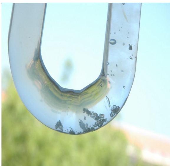
Fig. 2. Cadmium mercury thiocyanate crystals grown in a U-tube by gel method
