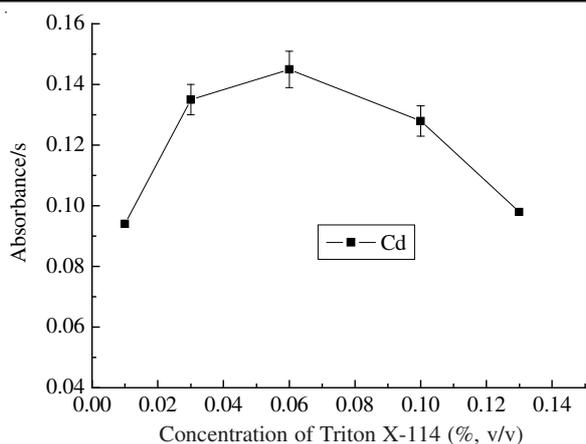
Fig. 3. Effect of Triton X-114 concentration on the analytical signal intensity of cadmium. Condition: Cadmium(II) standard solutions ( $0.5 \text{ ng mL}^{-1}$ ,  $6.00 \text{ mL}$ ),  $1.0 \text{ mL } 2.0 \%$  (w/v) ammonium pyrrolidine dithiocarbamate, Triton X-114 concentration  $0.01\text{-}0.13 \%$  (v/v), pH 4.0, equilibrium temperature  $50 \text{ }^\circ\text{C}$  and incubation time  $15 \text{ min}$
