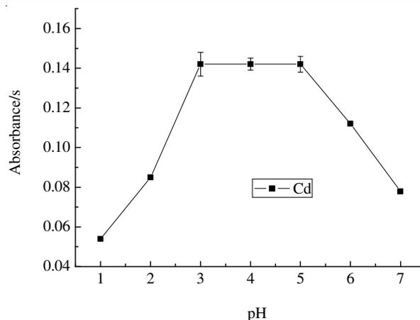
Fig. 1. Effect of pH on the signal intensity of cadmium in surfactant-rich phase. Condition: Cadmium(II) standard solutions (0.5 ng mL<sup>-1</sup>, 6.00 mL), 1.0 mL 2.0 % (w/v) ammonium pyrrolidine dithiocarbamate, 1.0 mL 1.0 % (v/v) Triton X-114, pH 1.0–7.0, equilibrium temperature 50 °C and incubation time 15 min
