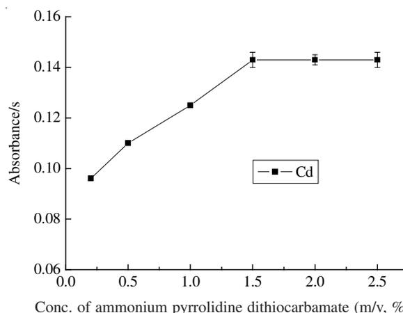
Fig. 2. Effect of ammonium pyrrolidine dithiocarbamate concentration on the analytical signal intensity of cadmium. Condition: Cadmium(II) standard solutions (0.5 ng mL<sup>-1</sup>, 6.00 mL), 1.0 mL 0.2–2.5 % (m/v) ammonium pyrrolidine dithiocarbamate, 1.0 mL 1.0 % (v/v) Triton X-114, pH 4.0, equilibrium temperature 50 °C and incubation time 15 min
