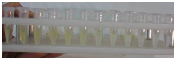
Fig. 2. Supernatant clarity of the 2-propanol (left) and zinc sulphate (right) modified, acetonitrile precipitation
