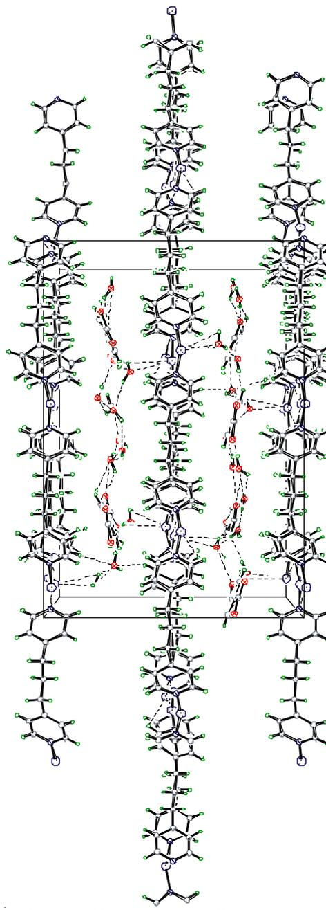
Fig. 2. Packing view of  $[\text{Ag}(\text{bpp})]_2(\text{BDC}) \cdot 8\text{H}_2\text{O}$  along *c* axis, showing the rich hydrogen bonds
