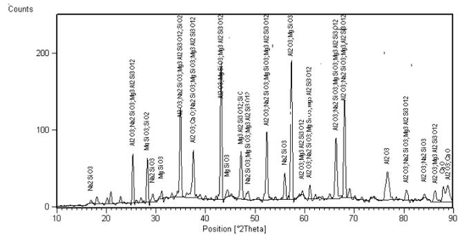
Fig. 5. Phase analysis of sample number 6
