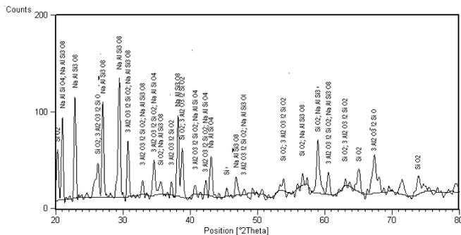
Fig. 3. Phase analysis of sample number 13
